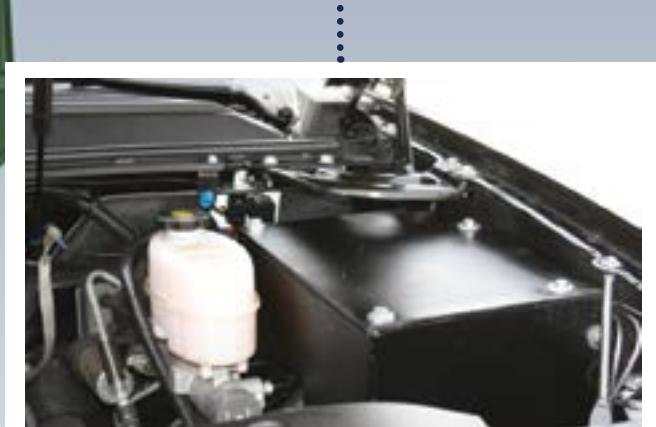
**ENGINE COMPARTMENT PROTECTION:** All armored vehicles come standard with armor protection for both engine side fenders, behind headlights, engine batteries, ECU and brake master cylinder. Full radiator protection is available as an upgrade option.
