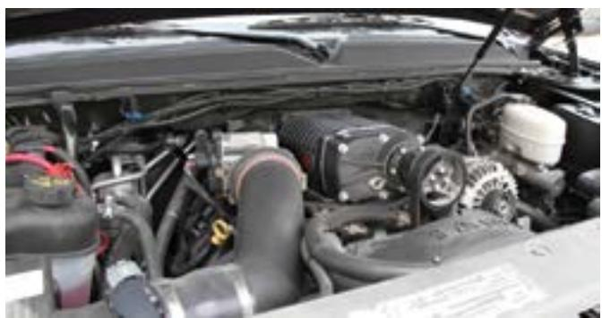
**POWER UPGRADES:** We offer a wide range of engine and power-train upgrades that allow each armored vehicle to reach our client's performance requirements. All power upgrades are designed such that the vehicle will retain its reliability. Upgrades include aftermarket superchargers, turbochargers, ECU retune, air intake and exhaust system upgrades, gear swaps and many other options.
