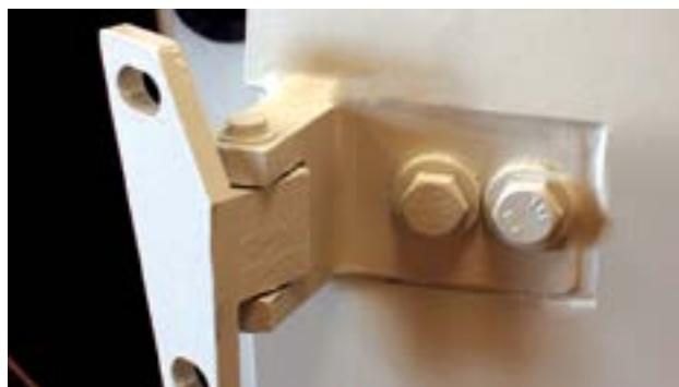
**DOOR RISER™ SYSTEM:** To support the weight of the armored door, IAG replaces all OEM door hinges with heavy duty steel billeted door hinges and installs our patented Door Riser™ system, a system that transfers the weight of the armored door onto the vehicle's frame when the doors are closed reducing the stress on the hinges.
