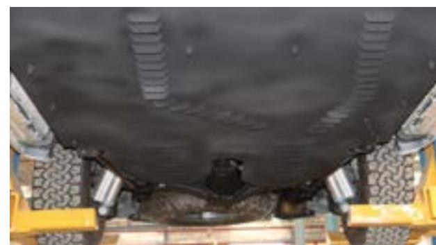
**FLOOR AND FUEL TANK PROTECTION:** All IAG vehicles come standard with blast protection against 2 x DM51 hand grenades. Optional upgrades are available for anti-tank mines, fragmentation grenades and other explosives. The fuel tank on every IAG vehicle is also protected against ballistic and explosive attacks.
