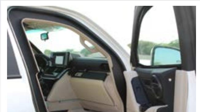
**DOOR OVERLAP:** all door apertures in every IAG vehicle is protected with 360 degree, full door overlap.
