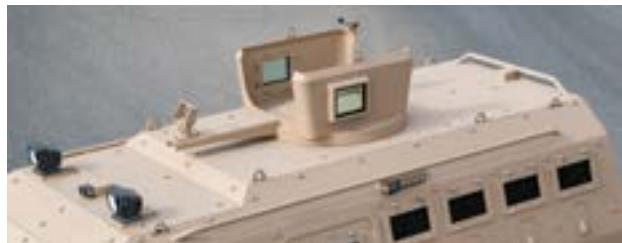
**ROOF PROTECTION:** All armored vehicles produced by IAG come with 90 degrees obliquity ballistic protection in the roof area, as opposed to only 45 degrees obliquity normally found in other armored vehicles. This design offers superior protection against potential attacks.
