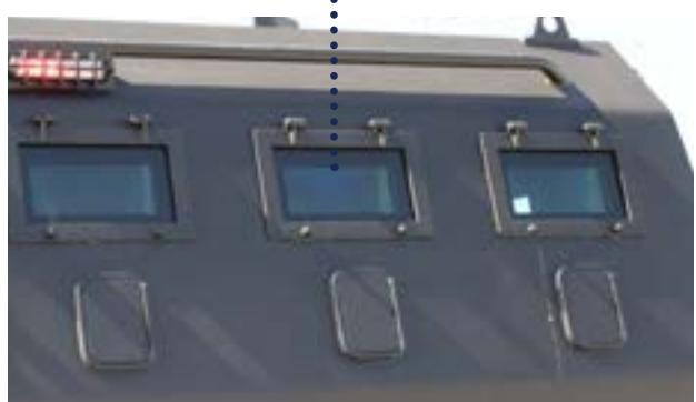
**CERTIFIED BALLISTIC GLASS:** By producing the ballistic glass in-house, IAG has the capability to custom fit and optimize each armor design for protection, cost, quality, weight and durability. All glass is pre-certified to provide multi-hit protection.
