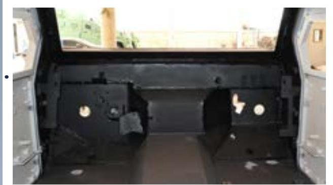
**SMARTARMOR™ FIREWALL** design with minimal number of pieces, derived from our BRV2009 VR7 certified vehicle, this firewall design provides protection against both ballistic and blast attacks.
